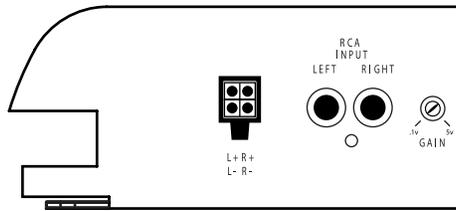
Located on the Input Panel, the objective of GAIN adjustment is to match the output of the source unit with the input of the amplifier. The output voltage of individual source units can vary. Some source units have an output of 200mV and others have 5 volts or more. To cater to these variations, the amplifier has an adjustable gain control that ranges from 100mV to 5 volts. Follow the steps below to set gains.
