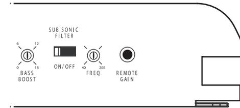
Note: If you are using the Remote Gain, make sure to take this into account during setup procedures of the subwoofer amplifier. You should set the system up with the Remote Gain plugged in, and with the level knob turned all the way down (counter-clockwise).
